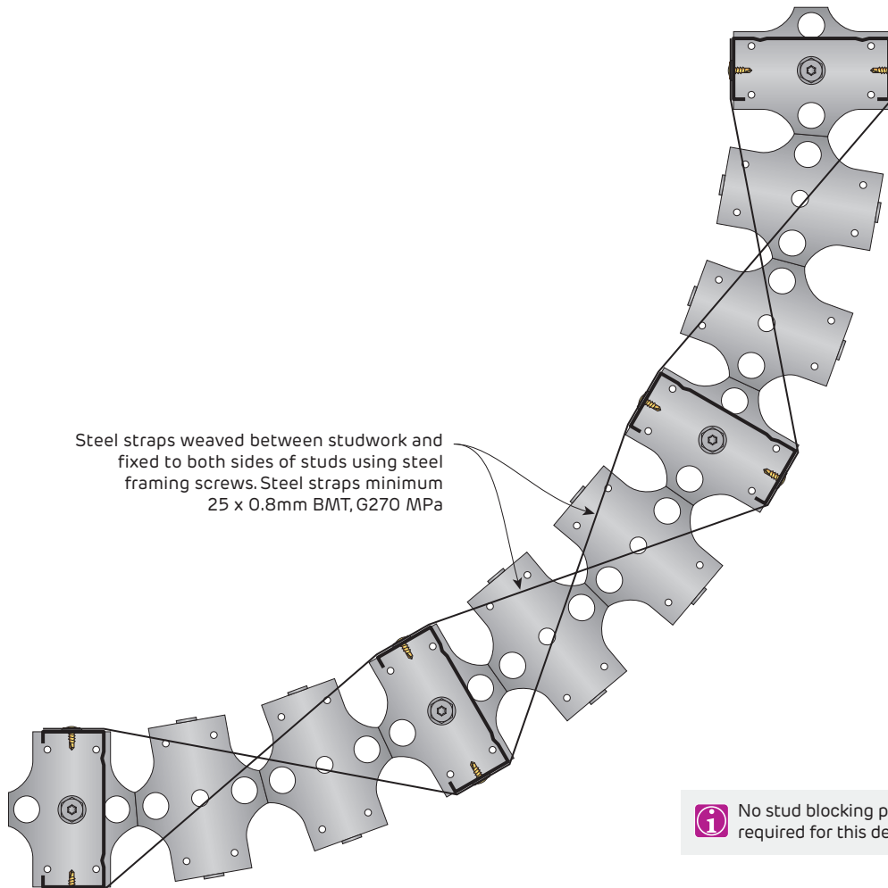
FIGURE 18 Strap Noggings for Curved Stud Walls Plan
