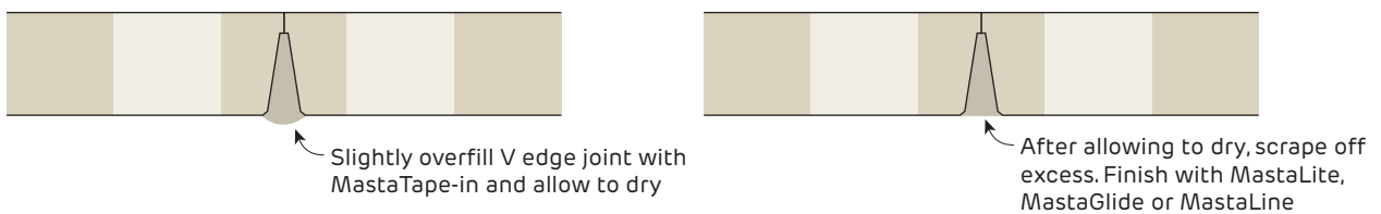
FIGURE 22 V Edge Jointing Section
