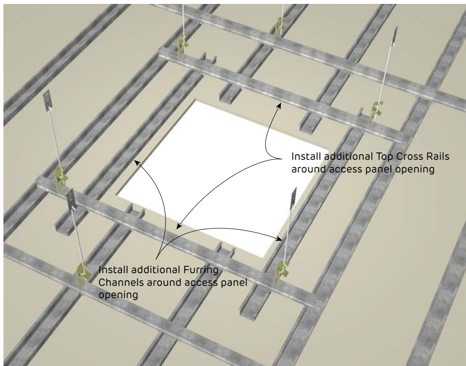
FIGURE 16 Createx Access Panel Framing Perspective
