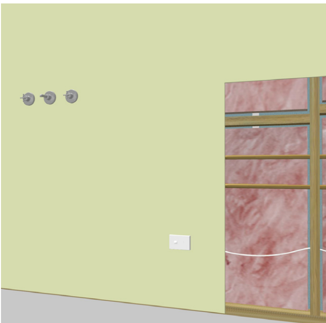
FIGURE 3 Services with Outer Layer of Plasterboard Installed
