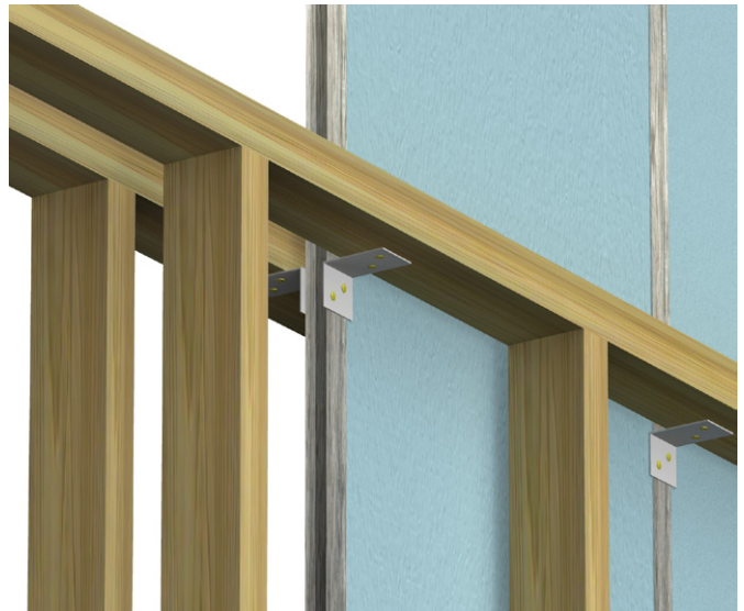
FIGURE 10 Aluminium Clips to H-studs and Frame
