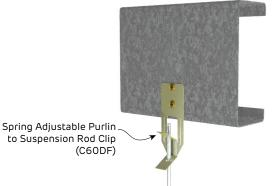
FIGURE 8 Spring Adjustable Direct Fix Clip to Purlin Perspective
