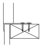
Fasten Fixing Tags to timber nogging with 10g timber screws
