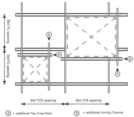
Extra suspension hangers will be required to support TCR ends and the additional TCR sections
