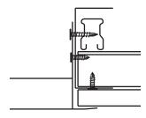
Fasten fixing tags to 64mm or 76mm trimming track and Top Cross Rail with 10g Tek screws
