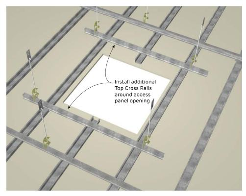
FIGURE 1 Chameleon Access Panel Framing Perspective
