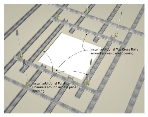
FIGURE 2 Chameleon Access Panel Framing Perspective
