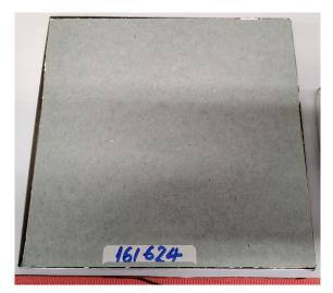
Watershield Plasterboard – 10 mm thickness sample
