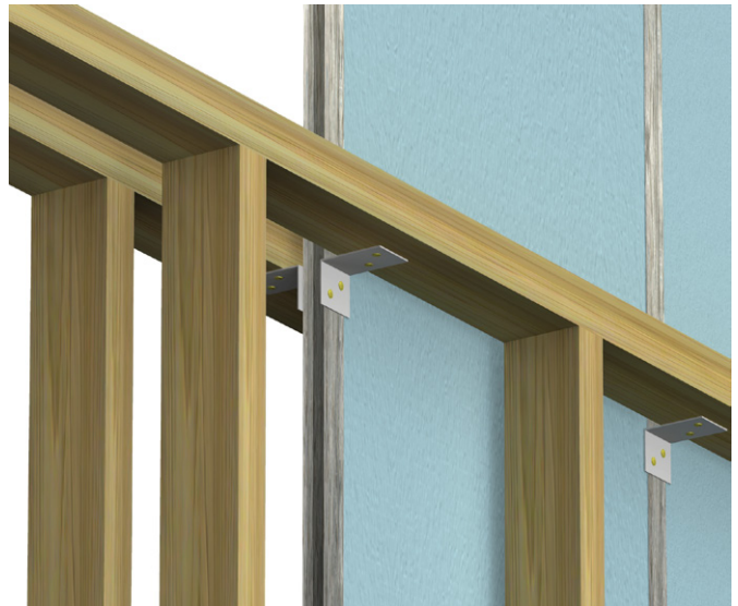
FIGURE 10 Aluminium Clips to H-studs and Frame
