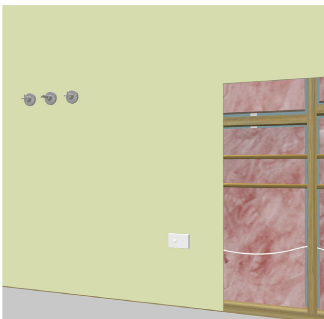
FIGURE 3 Services with Outer Layer of Plasterboard Installed
