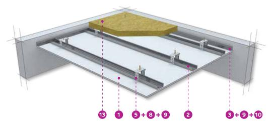
When making soffits to fasten the profiles with each other, use **FLAT HEAD** screws to prevent the deformation of the boards and cracking.
