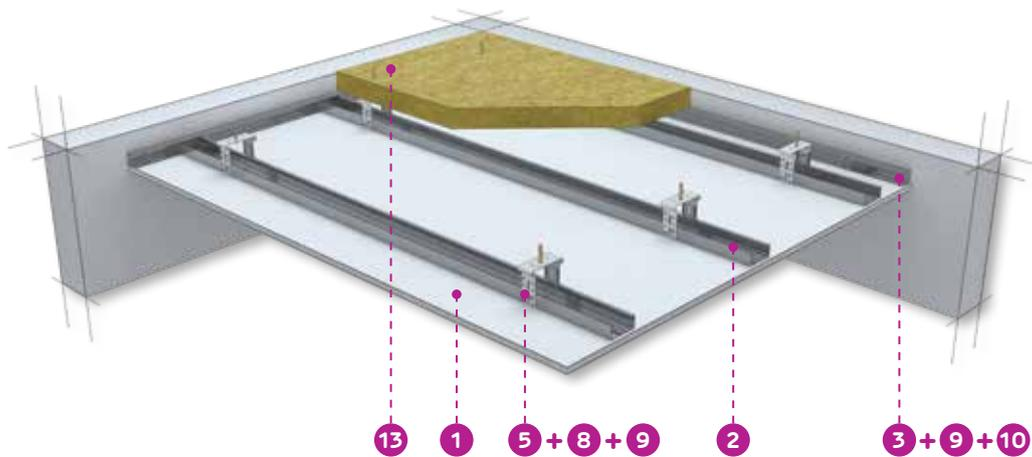
When making soffits to fasten the profiles with each other, use **FLAT HEAD** screws to prevent the deformation of the boards and cracking.
