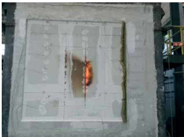
Image of the side not exposed to fire outside the test furnace
