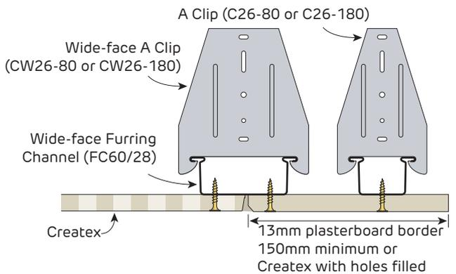
**FIGURE 30 Perimeter Detail - Border**
