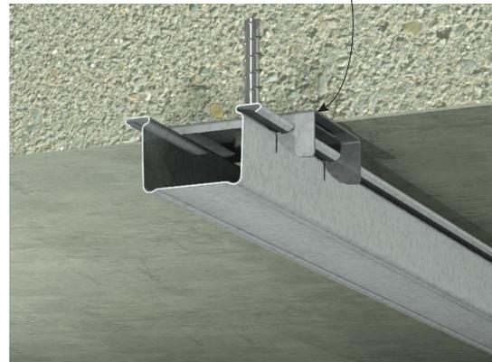
**FIGURE 4 Anchor Clip and Furring Channel Perspective**
