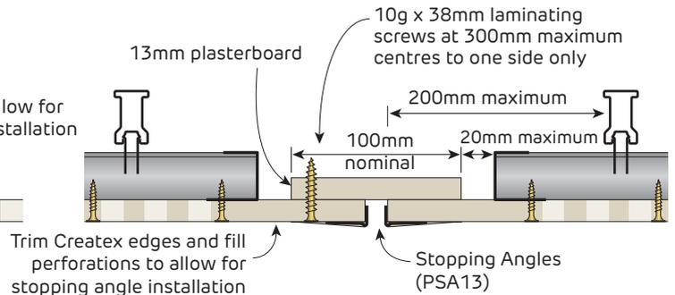
**FIGURE 27 Control Joint - Stopping Angles**
