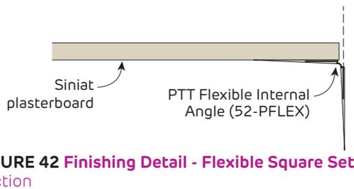
**i** Ceilings using a square set finishing detail have low tolerance for building movement and are more prone to cracking and joint peaking
