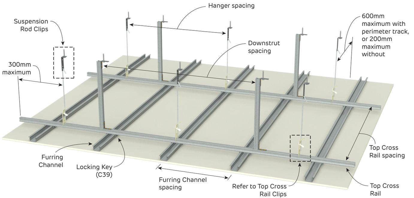
**FIGURE 6 Suspended Ceiling Frame with Downstruts**
