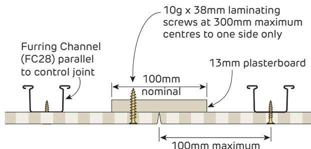
**FIGURE 28 Control Joint - Bare V Edges**
