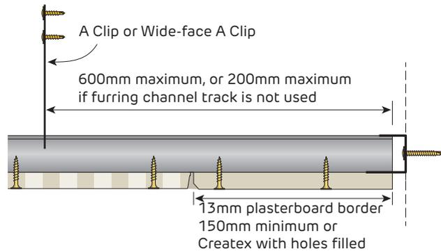
**FIGURE 31 Perimeter Detail - Border**
