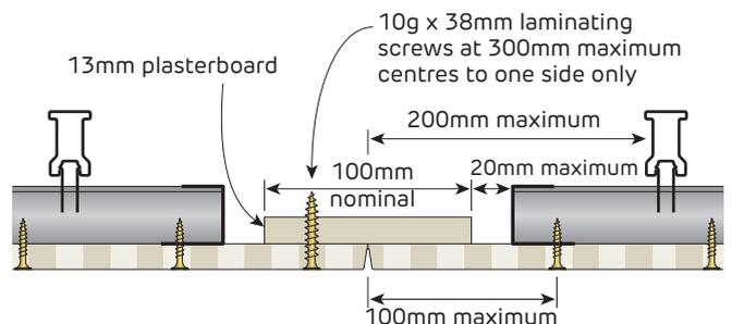
**FIGURE 29 Control Joint - Bare V Edges**
