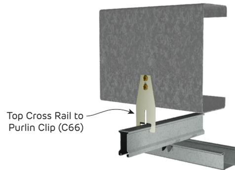
**FIGURE 10 Top Cross Rail Direct Fix Clip to Purlin**
