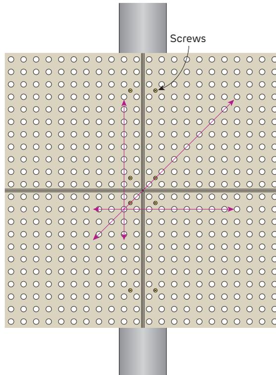
**FIGURE 19 Perforation Alignment**
