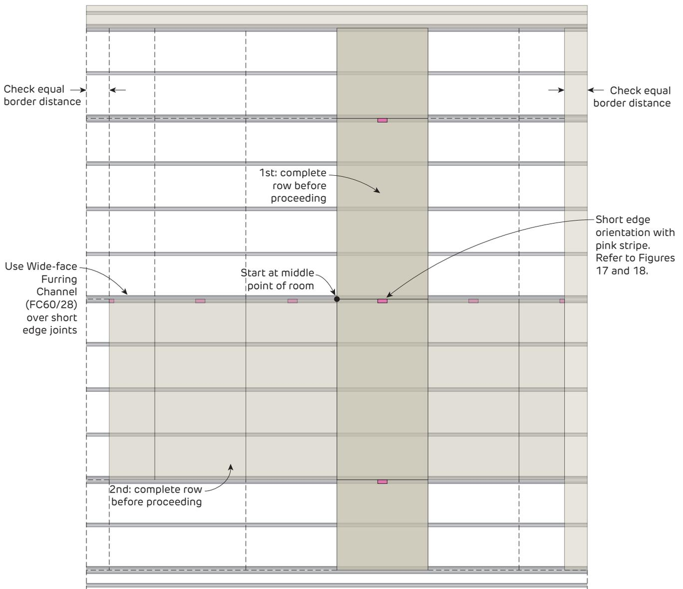
**FIGURE 16 Ceiling Layout Plan**
