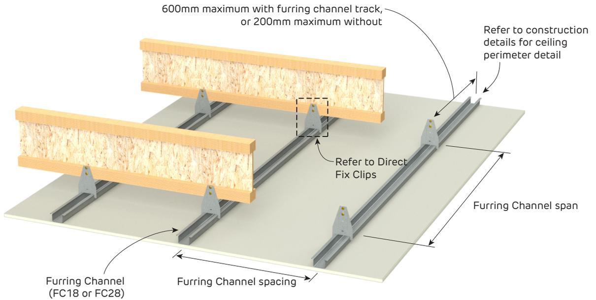
**FIGURE 1 Direct Fix Furring Channel Ceiling Frame**
