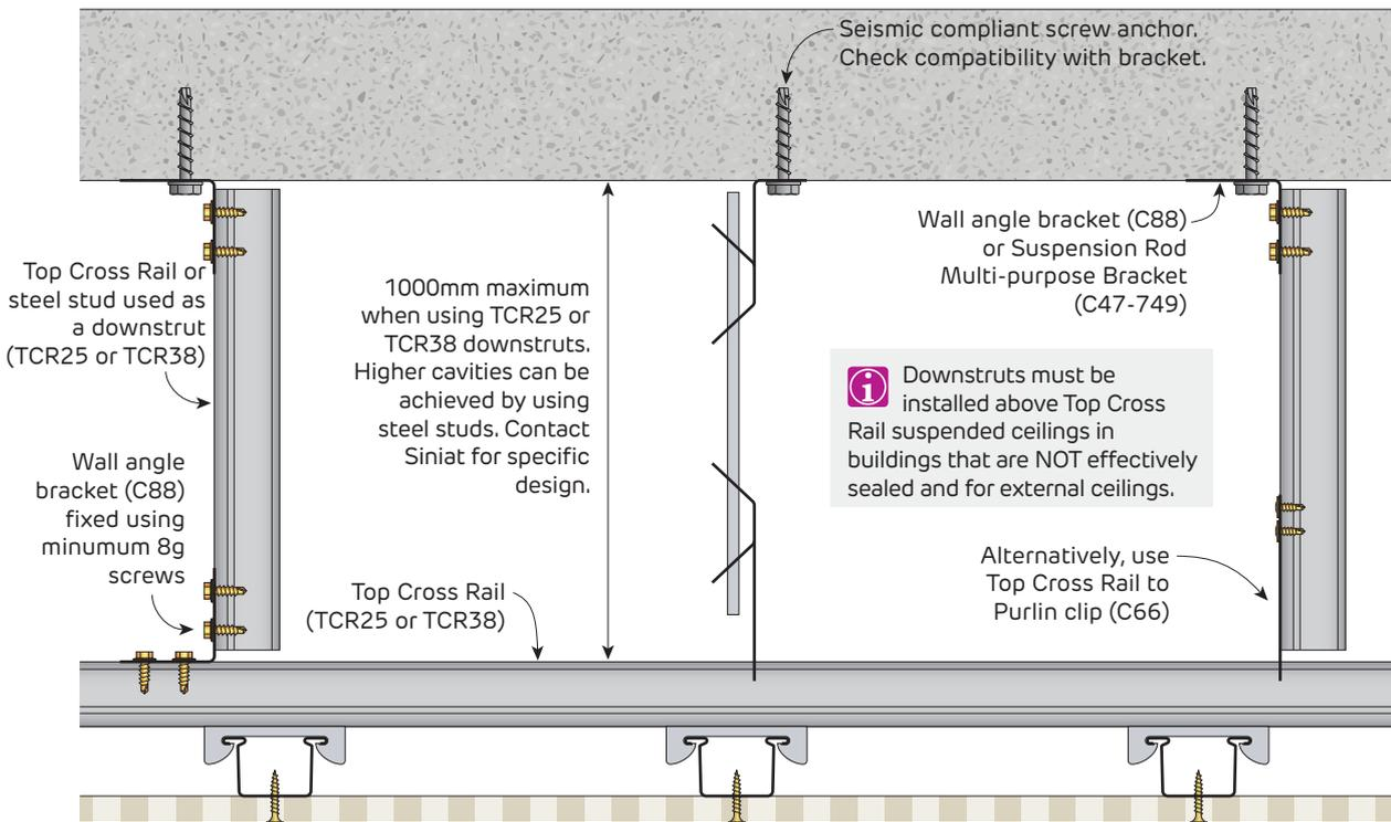
FIGURE 12 Downstrut Section
