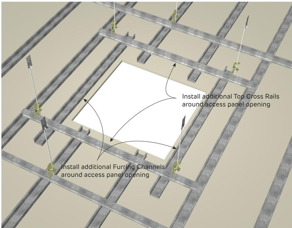
**FIGURE 15** Createx Access Panel Framing
