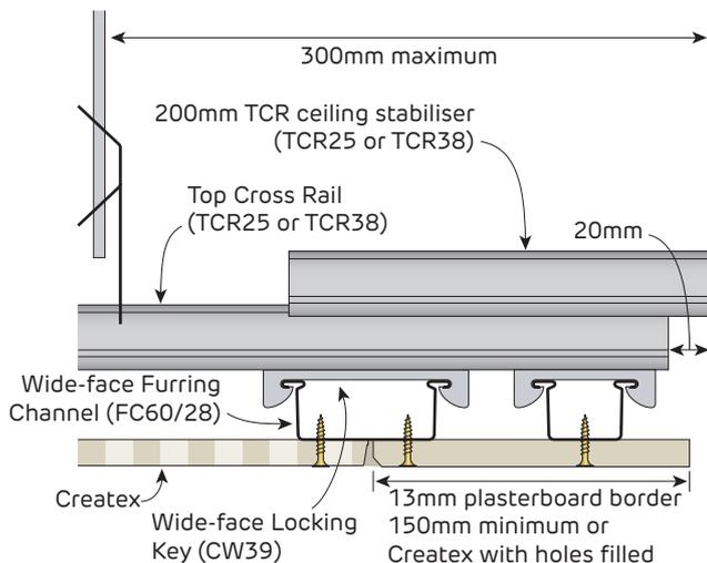
**FIGURE 32 Perimeter Detail - Border**
