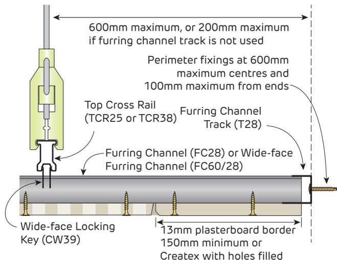
**FIGURE 33 Perimeter Detail - Border**
