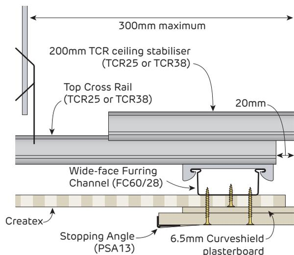
**FIGURE 35 Perimeter Detail - Proud Shadow Border**
