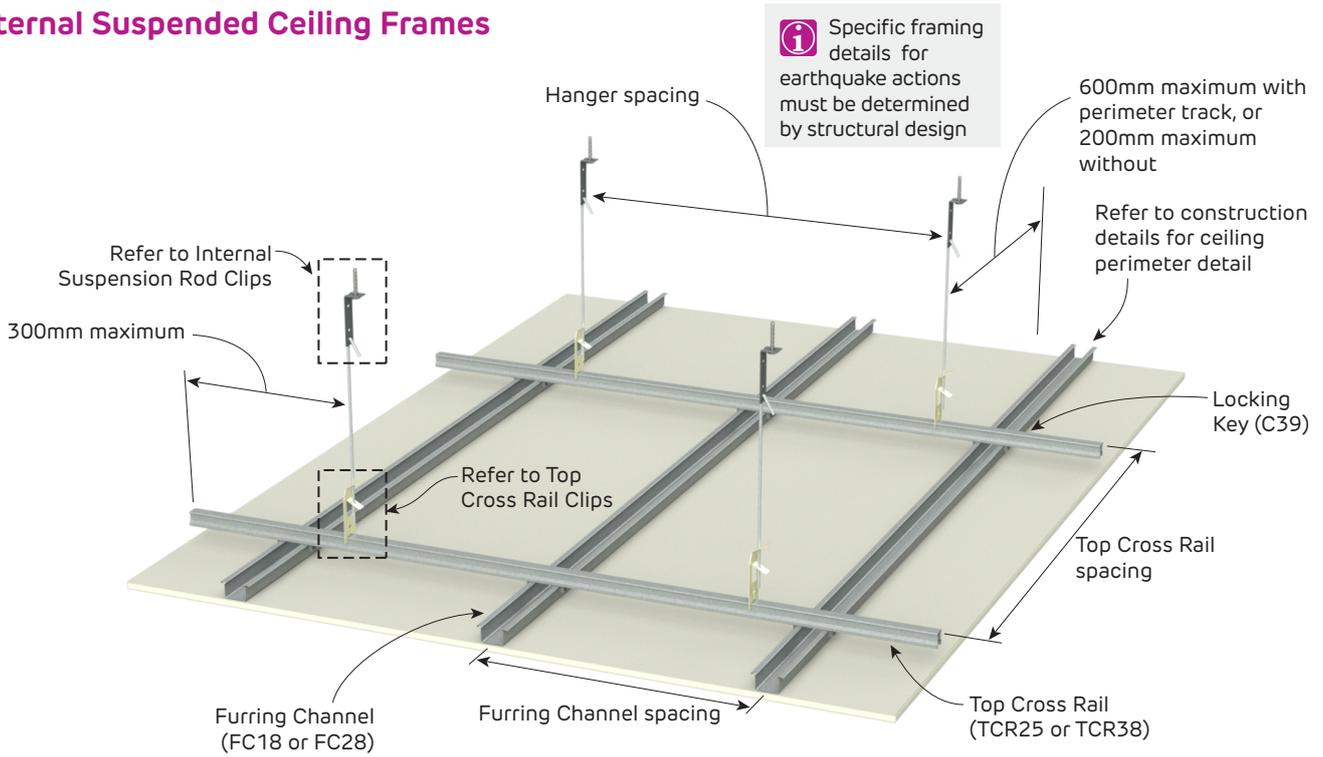
**FIGURE 5 Suspended Ceiling Frame**
