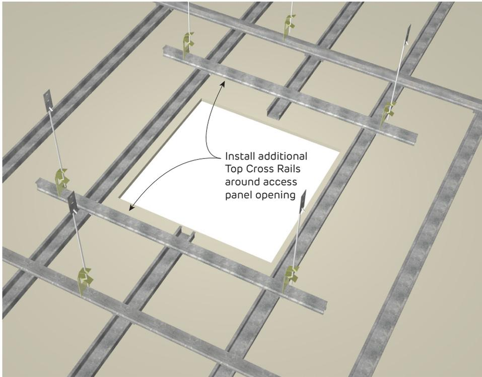
**FIGURE 14** Createx Access Panel Framing
