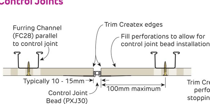
**FIGURE 26 Control Joint - Control Joint Bead**
