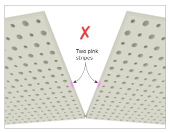
**FIGURE 18 Incorrect Short Edge Orientation**Perspective
