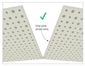
**FIGURE 17 Correct Short Edge Orientation**Perspective
