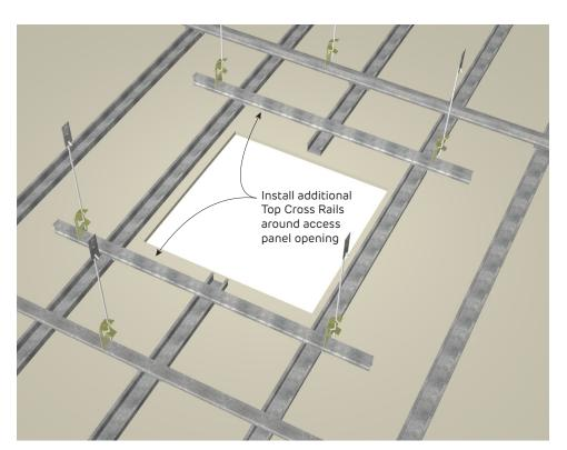
**FIGURE 14 Createx Access Panel Framing**Perspective
