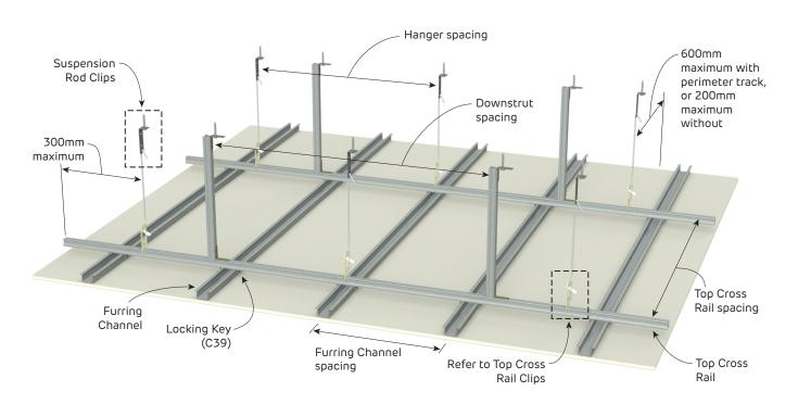
**FIGURE 6 Suspended Ceiling Frame with Downstruts**Perspective
