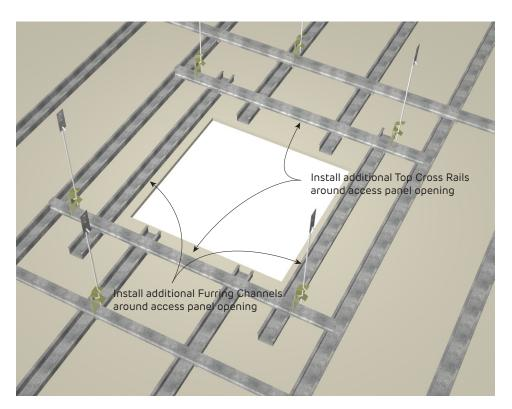
**FIGURE 15 Createx Access Panel Framing**Perspective
